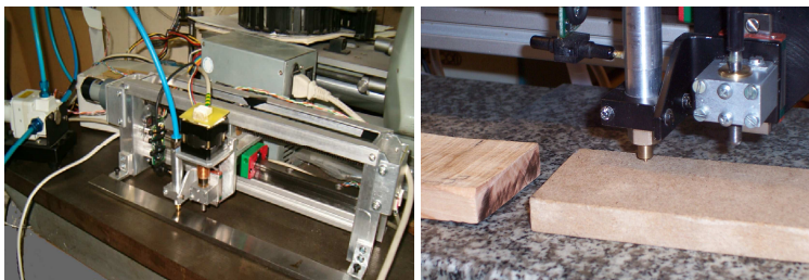
Fig. 2. Air gauge in the scanning device for contour and waviness measurement.
